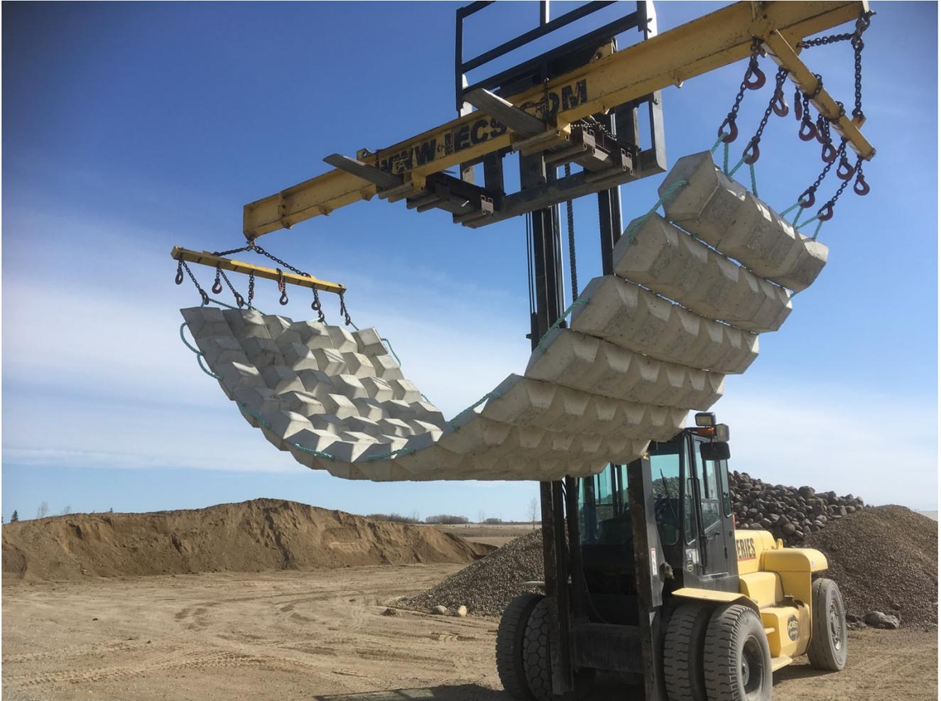
CC60M is a very viable solution for submerged hard armored applications such as pipeline protection and scour protection. With a centered cabling structure and a trapezoidal base to each block, the system is designed to be extremely flexible in both upward and downward directions. CC60 is an effective alternate to traditional methods such as rock armoring, sand and grout bags, structural concrete, and other hard armoring systems.
